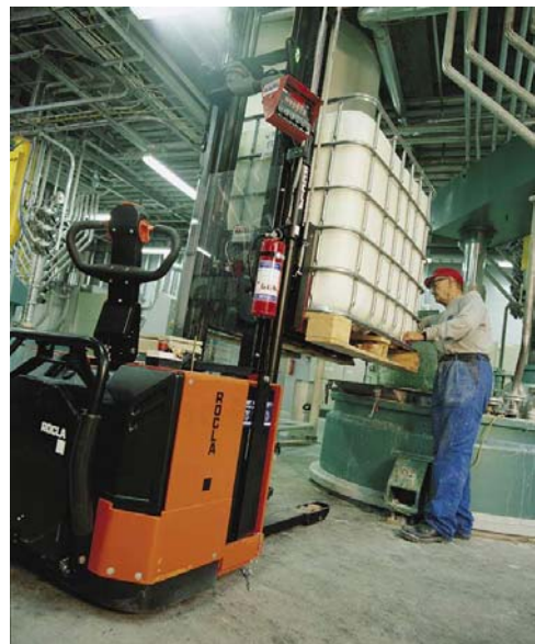
Dosing and filling going from containers, with a weighing system on the stacker
