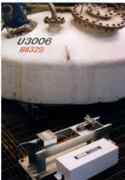
Close-up of conversion kit for mechanical vessel weighing system, showing load cell and other internal parts
